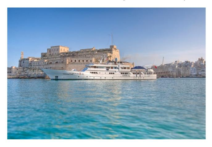
The long-range Navetta motoryacht 53-meter is a twin-screw displacement motor yacht built at the German Husumer Schiffswerft shipyard. Originally launched at a length of 37 meters, she has since undergone two extensions, first in 1984 and then in 2001, reaching her current impressive size.
